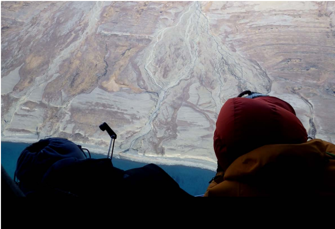
Figure 1. Acquisition of oblique stereo-images using two handheld cameras by taken photos out of the open Air Greenland B212 helicopter door at 1000 m altitude.
